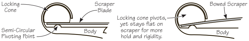
Figure 2: Bowing the scraper blade.
